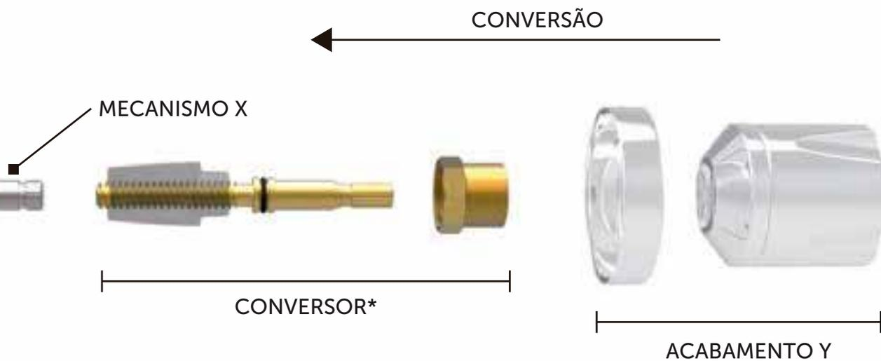
INSTALAÇÃO PARA CONVERSORES\* COMPOSTOS POR CASTELO E/OU HASTE CONVERSORA COM SISTEMA DE GAVETA
